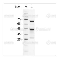
SDS-PAGE of purified antibody under reduced condition. Lane M: Protein marker Lane 1: Normal Chicken IgY (2 µg, reduced)
